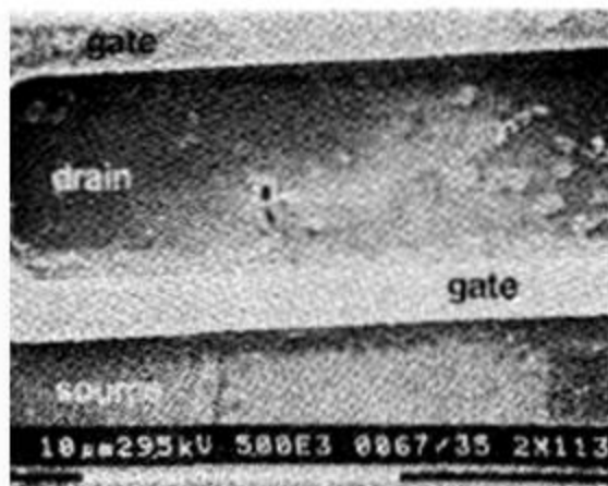
Fig.8. SEM photograph of a contact hole in the drain diffusion region of an NMOS output transistor showing a hole due to contact spiking.
