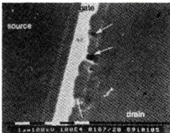
Fig.6. SEM photograph of an NMOS transistor, after partial n + polysilicon etch to expose the gate oxide, showing gate-oxide damage .
